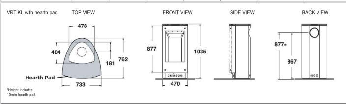
Dimensions shown above are in millimetres and for reference only. Refer to installation manual for detailed specifications on installing this product. Heat & Glo reserves the right to update units periodically. The flame and ember appearance may vary based on the type of fuel burned and the venting configuration used. Actual product appearance, including flame and logs may differ from the actual product.
