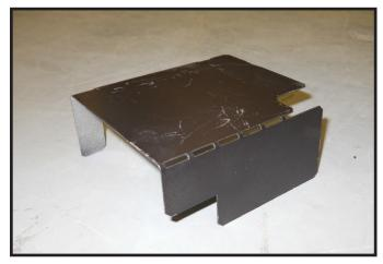
Figure 14.3 Heat Shield Bends
