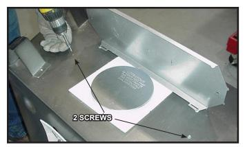
Figure 9.3 Replace the two screws as shown.
