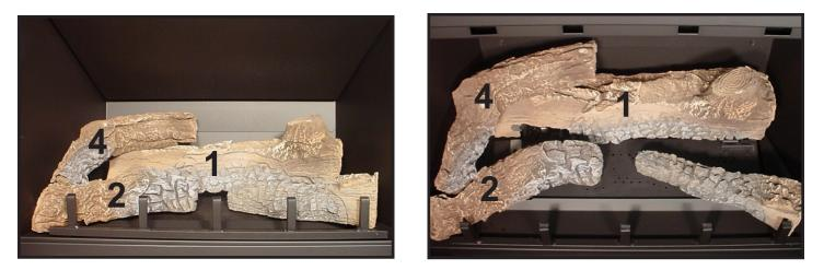
LOG #4 (SRV530-716): Place the left end of log #4 in the groove on log #2 and the right end on log #1 as shown.
