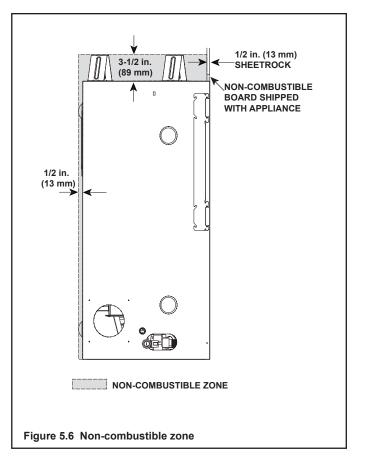
If joints between the finished walls and the heater surround (top and sides) are sealed, a 149 °C (300 °F) minimum sealant material must be used. These joints are not required to be sealed. Only non-combustible material (using 149 °C (300 °F) minimum adhesive, if needed) can be applied as facing to the heater surround. See Figure 5.7.
