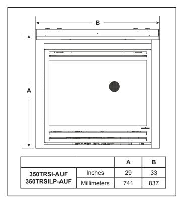
Figure 13.3 Noncombustible Facing Diagram
