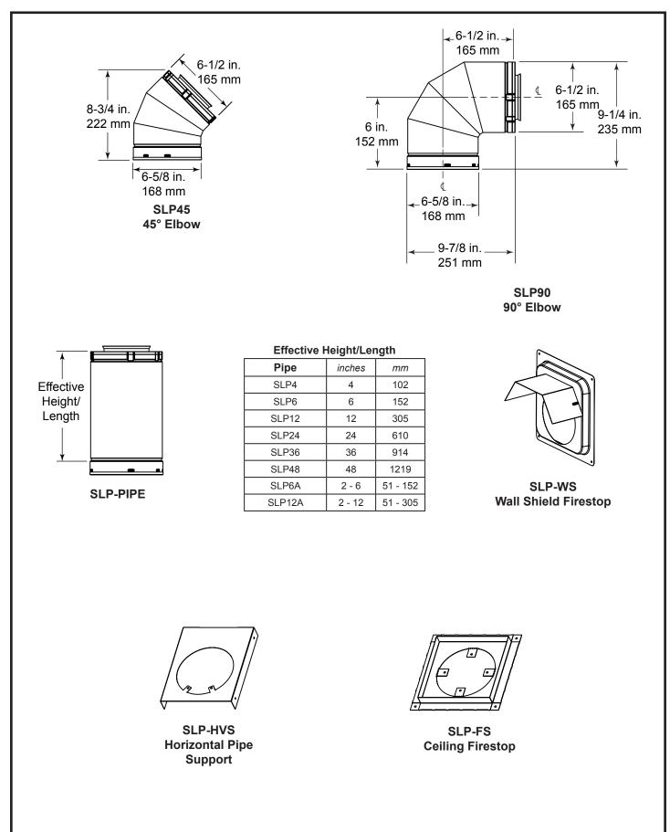
Figure 16.6 SLP Series Vent Components
