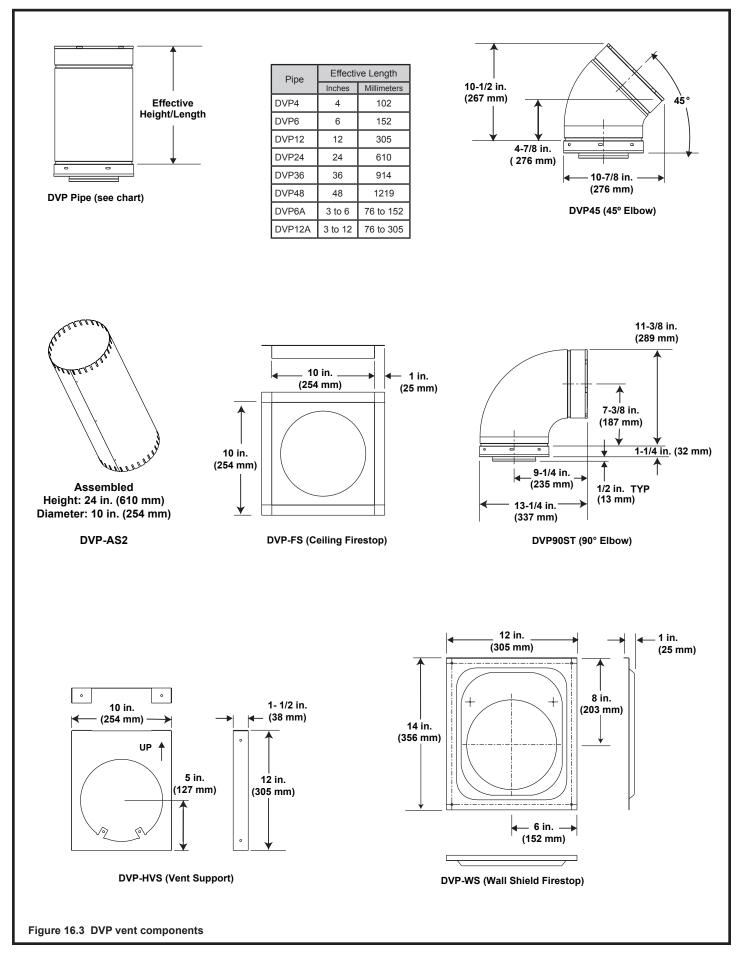
Note: Heat shields MUST overlap by a minimum of 1-1/2 in. (38 mm). **The heat shield is designed to be used on a wall 4 in. to 7-1/4 in. (102 mm to 184 mm) thick.** If wall thickness is less than 4 in. (102 mm) the existing heat shields must be field trimmed. If wall thickness is greater than 7-1/4 in. (184 mm) a DVP-HSM-B will be required.
