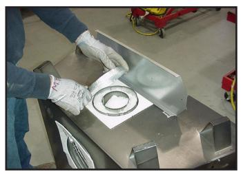
Figure 9.4 Remove the seal cap.
