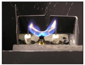
Figure 3.1 IPI Pilot Flame Patterns
