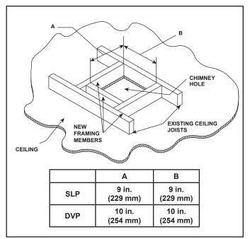
Figure 10.14 Hole and New Framing Members
