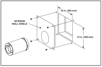
Figure 10.13 Flue Pipe & Firestop
