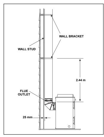
Figure 10.12 Installing Support Brackets
