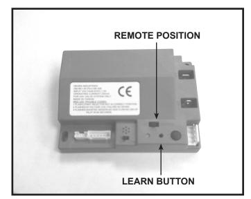
Figure 12.9 Programming RC300AU
