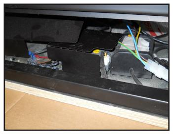
Figure 14.4 Heat Shield Placement
