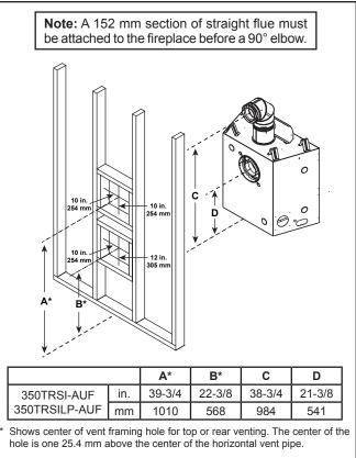
Figure 8.2 Wall Penetration
