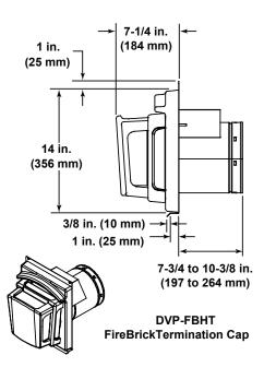
Figure 16.4 DVP vent components
