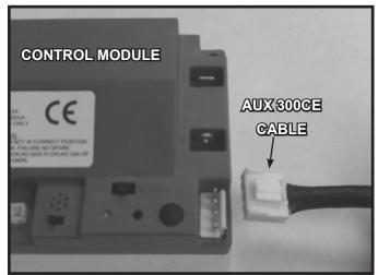
Figure 12.7 AUX 300 module installation
