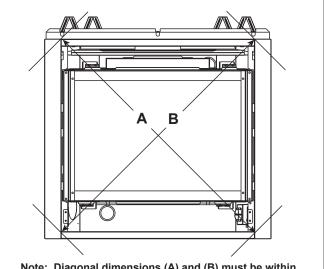
Note: Diagonal dimensions (A) and (B) must be within 1/4 in. (6 mm) of each other.
