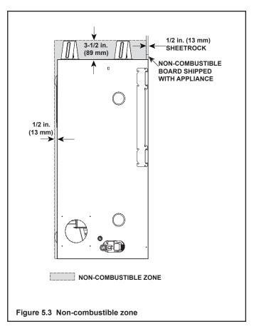
If joints between the finished walls and the heater surround (top and sides) are sealed, a 149 °C (300 °F) minimum sealant material must be used. These joints are not required to be sealed. Only non-combustible material (using 149 °C (300 °F). minimum adhesive, if needed) can be applied as facing to the heater surround. See Figure 5.4.
