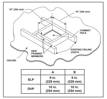
Figure 10.14 Hole and New Framing Members
