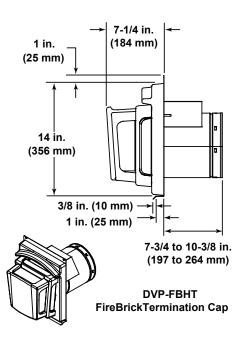
Figure 16.4 DVP vent components
