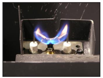
Figure 3.1 IPI Pilot Flame Patterns
