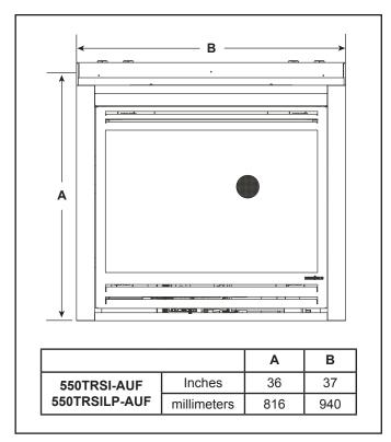
Figure 13.3 Noncombustible Facing Diagram
