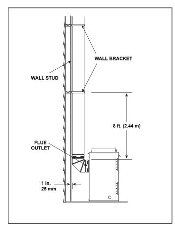
Figure 10.12 Installing Support Brackets
