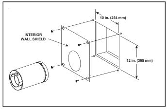
Figure 10.13 Flue Pipe & Firestop
