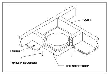
Figure 10.15 Ceiling Firestop (Ceiling Side)
