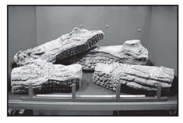
**LOG #4 (SRV327-704):** Place the bottom left corner of log #4 behind log #2 and rest its top right corner on log #1.
