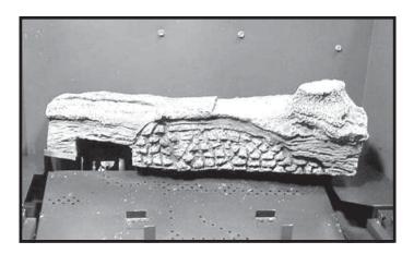
**LOG #1 (SRV327-701):** Place log #1 in the back of the heater, locating it's slot on the right over the protruding tab. The left end of the log is positioned by the two bend up tabs shown in Photo A.
