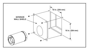
Figure 10.12 - Flue Pipe & Firestop
