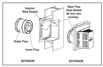
Figure 10.16 - Venting through the Wall
