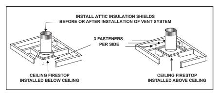
Figure 8.4 - Installing the Attic Shield
