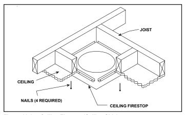
Figure 10.14 - Ceiling Firestop (Ceiling Side)
