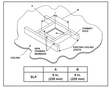
Figure 10.13 - Hole and New Framing Members
