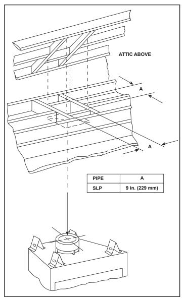
Figure 8.3 - Installing Ceiling Firestop
