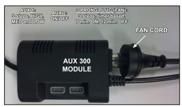
Figure 12.9 - Plug Fan into AUX300CE Module
