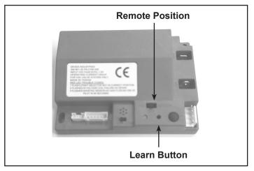
Figure 12.10 - Programming RC300AU
