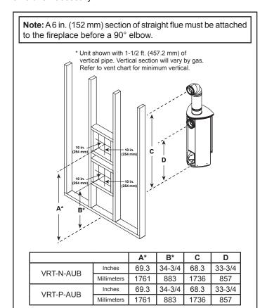
Shows center of vent framing hole for top or rear venting. The center of the hole is one 1 in. (25.4 mm) above the center of the horizontal vent pipe.
