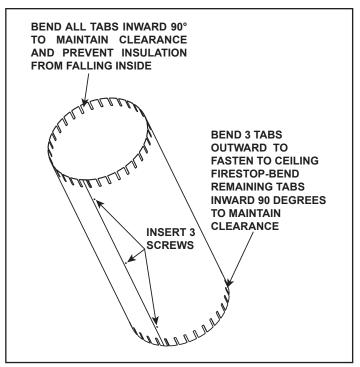
Figure 8.5 - Attic Insulation Shield
