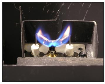
Figure 3.1 - IPI Pilot Flame Patterns
