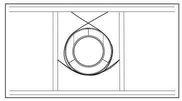
Figure 10.6 - Securing Horizontal Pipe Sections
