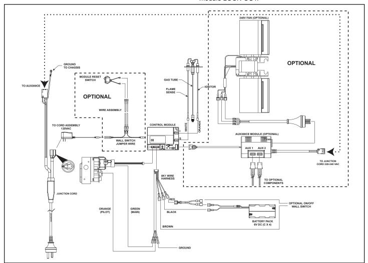
Figure 12.1 - IPI Wiring Diagram /RC300AU
