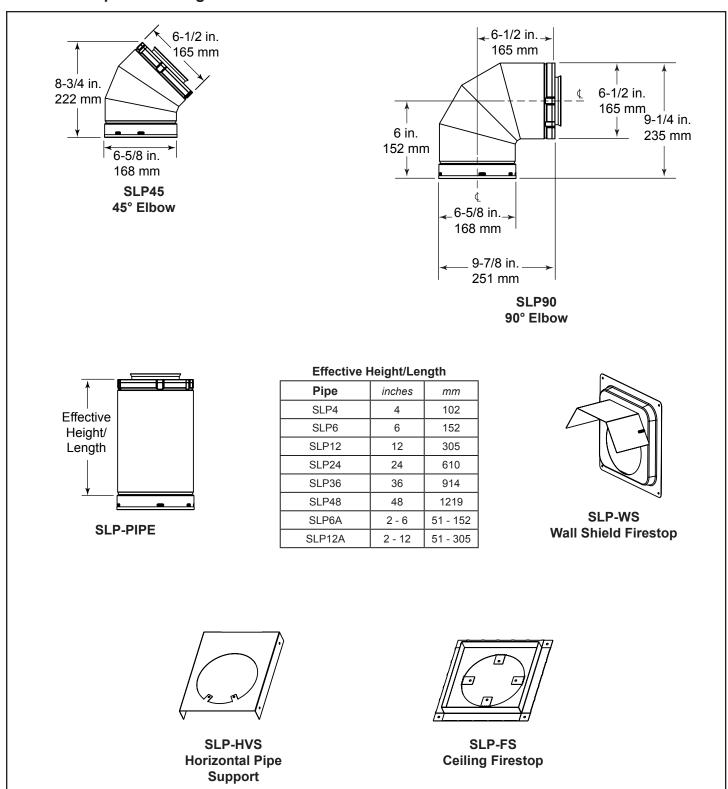
Figure 14.3 - SLP Series Vent Components
