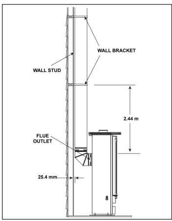
Figure 10.11 - Installing Support Brackets
