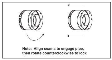
Figure 10.1 - Adding Venting Components
