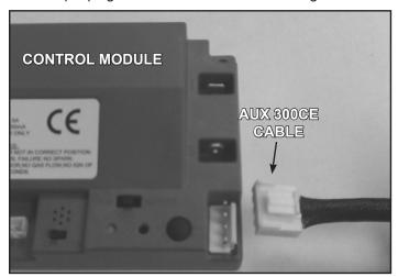
Figure 12.8 - AUX 300 module installation
