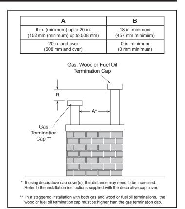
Figure 6.2 - Staggered Termination Caps
