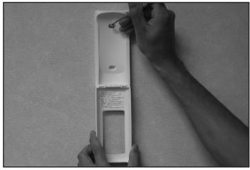
Figure 12.5 - Mounting Remote Control Housing
