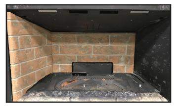
Figure 7. Left Refractory Installed
