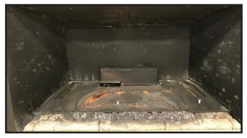
Figure 4. Base Refractory Installed
