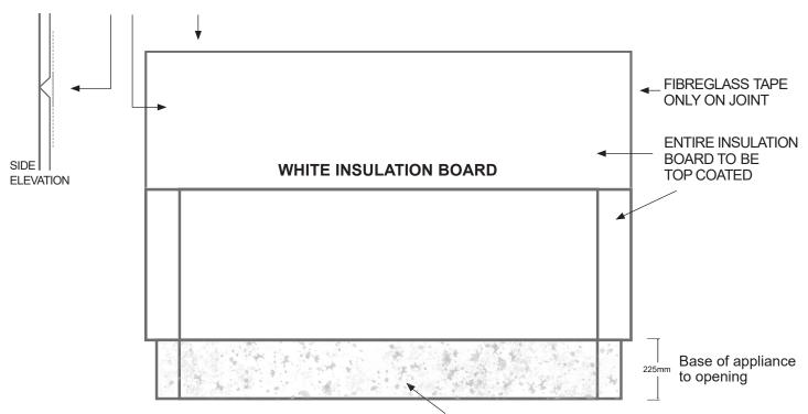
This area should be covered with finishing materials. Plaster channel on upper lip of lower panel.
