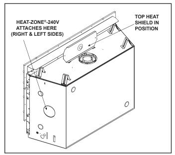
Figure 6.2 Top Heat Shield in Position and Heat-Zone<sup>®</sup>-240V Locations
