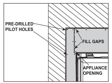
Figure 10.1 Install Non-Combustible Board
