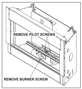
Figure 9.2 Burner Removal
