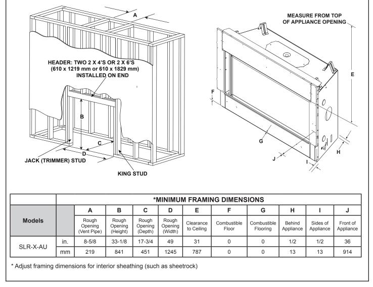
Figure 3.4 Clearances to Combustibles
