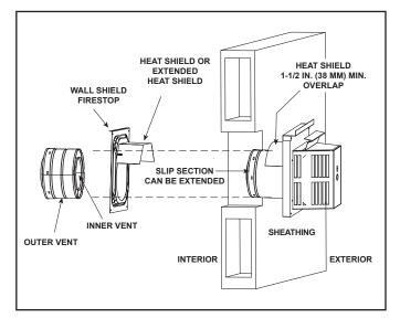
Figure 7.13 Venting Through the Wall
