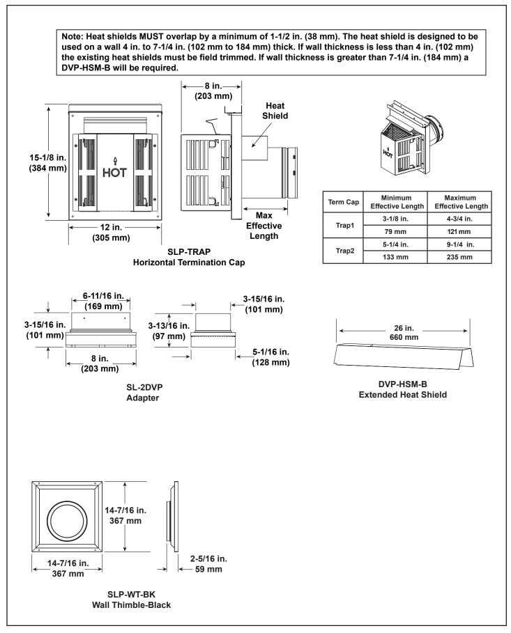
Figure 12.2 SLP Series Vent Components
