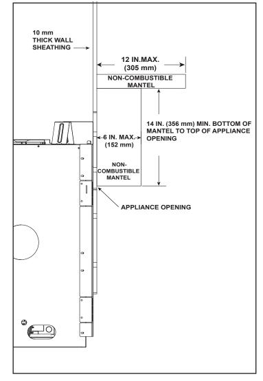
Figure 10.4 Clearances To Non-Combustible Mantels Or Other Non-Combustibles Above Appliance
