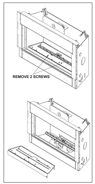
Figure 9.1 Base Pan Removal
