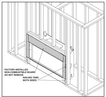
Figure 6.3 Proper Positioning, Leveling And Securing Of Appliance
