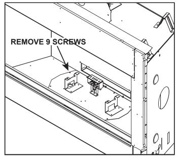
Figure 9.3 Remove Valve Plate
