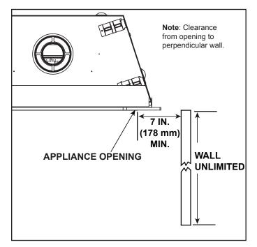
Figure 10.6 Combustible or Non-Combustible Mantel Leg or Wall Projections - Unlimited Wall Length (Acceptable on both sides of opening)
