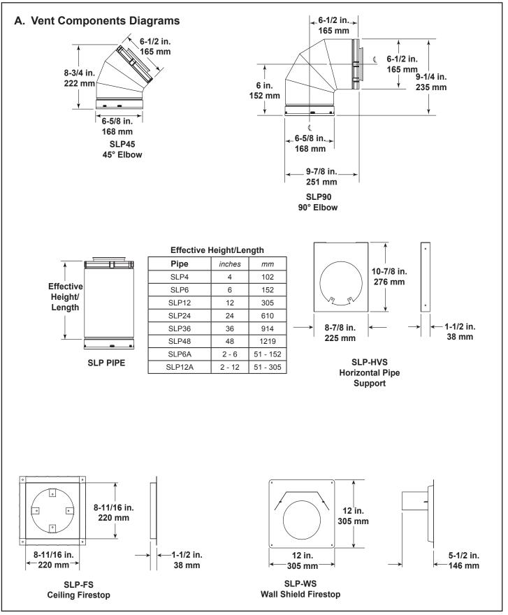
Figure 12.1 SLP Series Vent Components
