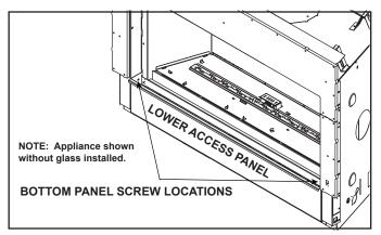
Figure 8.1 Lower Access Panel Location
