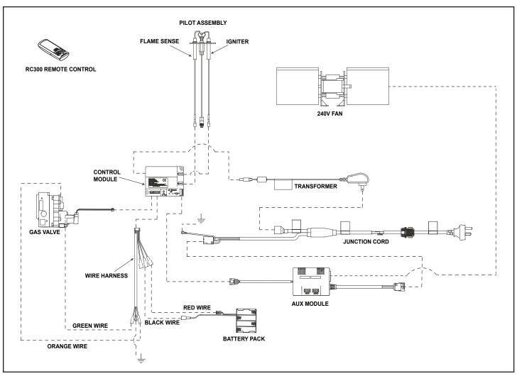
Figure 8.3 IntelliFire™ Plus Wiring Diagram with Remote
