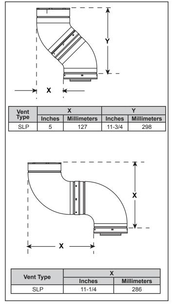
Figure 4.5 Vertical and Horizontal Offset for SLP Elbows
