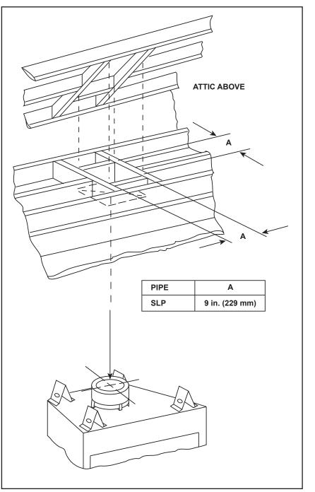
Figure 5.3 Installing Ceiling Firestop
