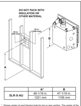
Shows center of vent framing hole for top or rear venting. The center of the hole is 1 in. (25 mm) above the center of the horizontal vent pipe.
