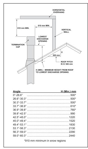
Figure 7.9 Minimum Height From Roof To Lowest Discharge Opening
