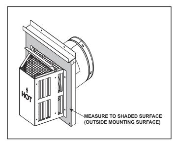
Figure 4.6 Measure to Outside Mounting Surface
