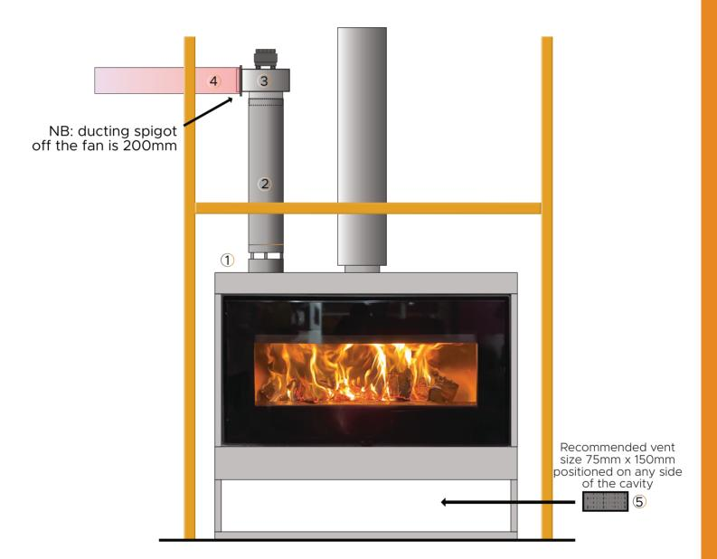
Ducting must be installed by a licensed professional to AS 4254.1-2012 'Ductwork or air-handling systems in buildings Flexible Duct 'compliance.
