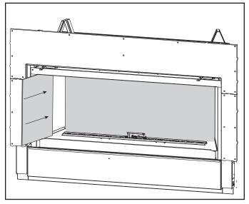
Figure 4. Placement of Side Glass Panel
