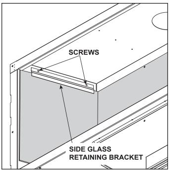
Figure 5. Placement of Side Glass Bracket - 32 Inch Models
