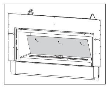
Figure 2. Placement of Rear Glass Panel
