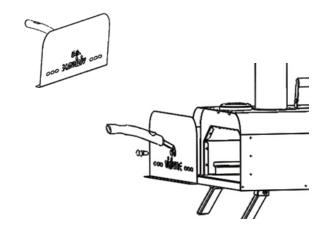
4. Attach handle to pellet burn basket with 2 x bolt and 2 x nut. Nut goes to inside of basket.
