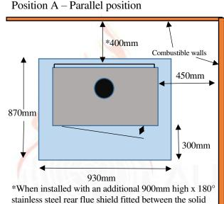
casing and the active flue the rear wall clearance can be
