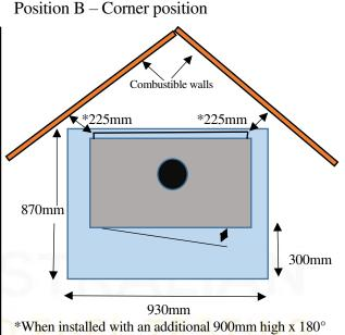
stainless steel rear flue shield fitted between the solid casing and the active flue.
