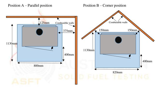
Figure 1 – Clearance Diagram
