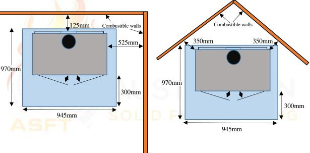
Figure 1 – Clearance Diagram
