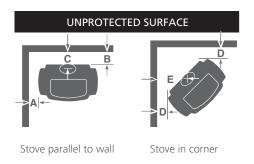
Minimum floor protection:1100mm (D) x 945mm (W). See manual for corner floor protection sizes and diagrams. Default flue with Decromesh or single rear heat shield only. Solid flue only permitted with Visionline Safety Vent Air Flue installation.
