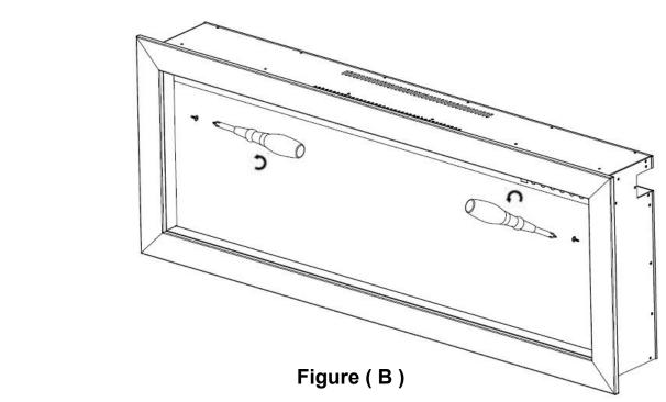
**STEP 2. Place** the fireplace to a **soft clean place**. using the screw driver to take off the **TWO** screws in both sides. **Figure (B)**
