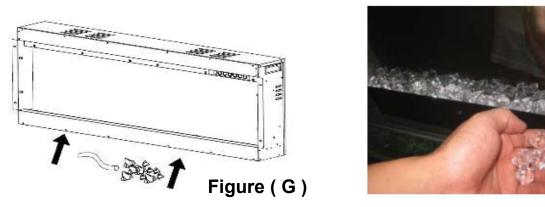
**STEP 7.** After Placing the decorative crystals and Drift log pieces on the designed slot and even with them from side to side . Move and screw back the glass panel and metal trim. (Repeat as **Fig B,C,D,E**)
