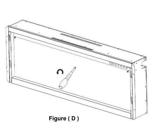
**STEP 4.** Using the screw driver to take off the 2 screws as above **Figure (D)**, have two adults to take out the glass panel **Figure (E)** and move it to a clean soft place to avoid the scratching. **NOTICE:** If you prefer initial ember bed, you can skip this step.
