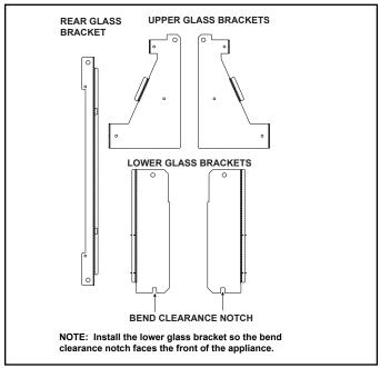
Figure 1. Metal Components - Components Shown Bent
