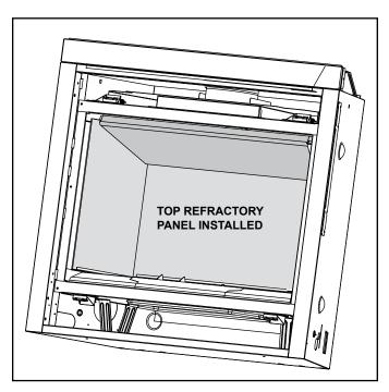
Figure 12. Top Refractory Panel
