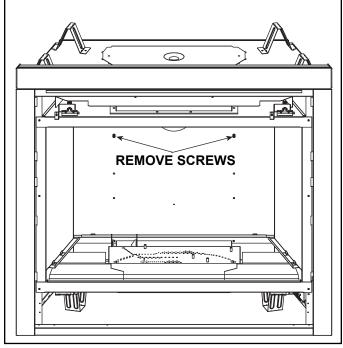
Figure 5. Remove Screws
