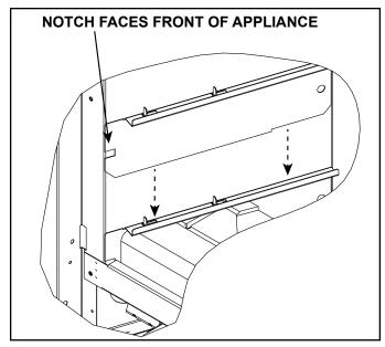
Figure 3. Install Lower Glass Bracket (Left Side Shown)
