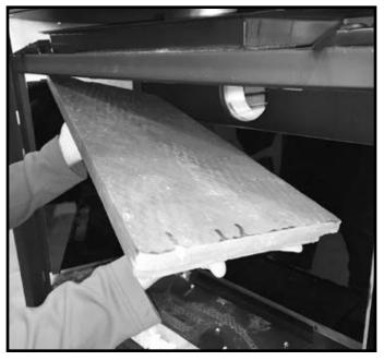
Figure 11. Install Top Refractory Panel
