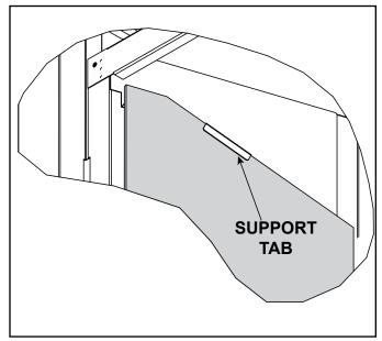
Figure 9. Install Left Glass Panel
