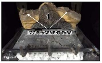
Figure 6 shows the log placement tabs located on the top of Log # 1. The tabs will be mated with the slots located on the bottom of Log #2 and Log #3 (see Figure 7). Log #2 and Log #3 also have grooves that allow the logs to be seated properly on the grate (see Figure 7). Hold Log #1 upright while placing Log #2.
