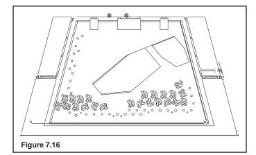
Apply 15 mm size pieces sparingly along ports as shown. Do not block ports.
