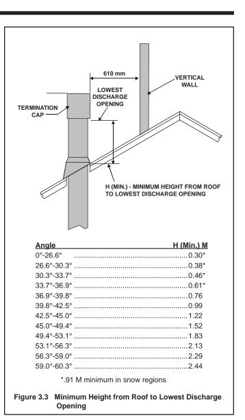
Figure 3.3 specifies minimum flue heights for various pitched roofs.
