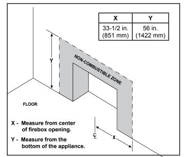
Figure 3.8 Non-Combustible Facing Requirement
