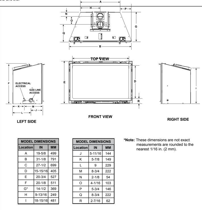
\*Note: Location G is the appliance depth measurement, for installation depth reference Location E on Figure 3.6.
