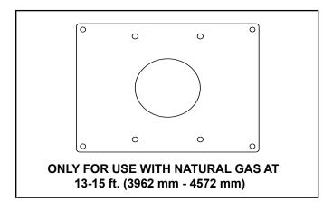
Figure 5.6 Natural Gas Restrictor Plate
