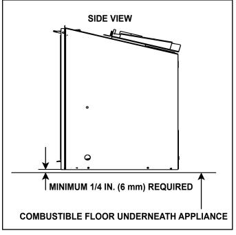
Figure 8.7 Solid Fuel Floor Clearance
