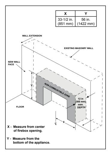
Figure 3.7 Minimum Non-Combustible Framing Requirement
