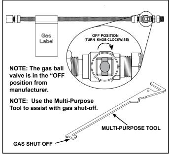
Figure 7.1 Gas Shut-off
