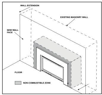
Figure 3.9 Non-Combustible Framing / Facing Requirement
