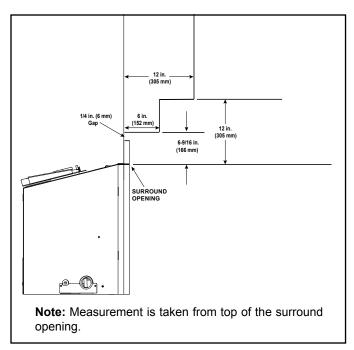
Figure 3.12 Minimum Vertical and Maximum Horizontal Dimensions- Non-Combustible
