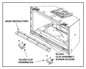
Figure 7.2 Glass Clip Assembly Removal
