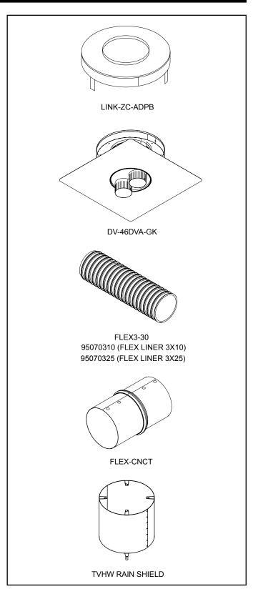
Figure 10.2 Direct Vent Flex Liner Accessory Kits
