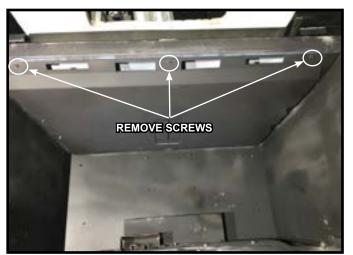
Figure 5.7 Remove Baffle Cover
