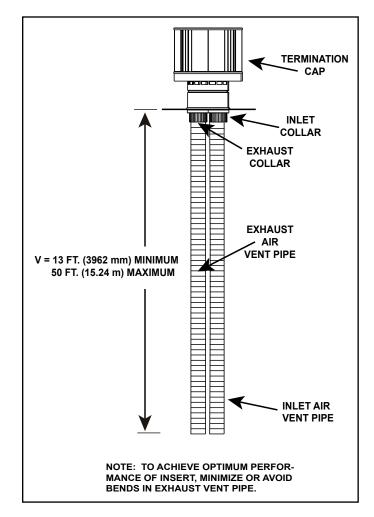
Figure 5.2 Min. / Max. Venting Requirement
