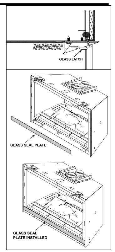
Figure 9.2 Glass Seal Plate and Glass Latch
