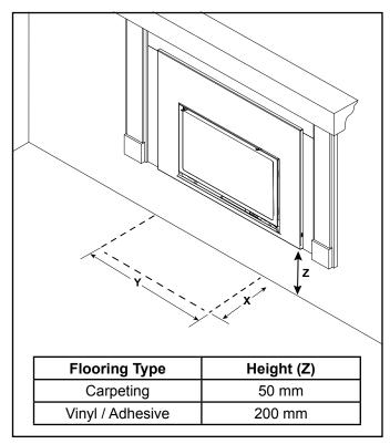
Figure 3.16 Hearth - Minimum Height for Vinyl / Adhesive or Carpeting Flooring
