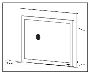
Figure 3.5 Minimum Required 1/2 in. (13 mm) Gap
