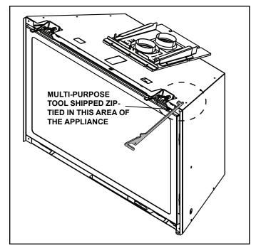
Figure 2.2 Multi-Purpose Tool shipping Location
