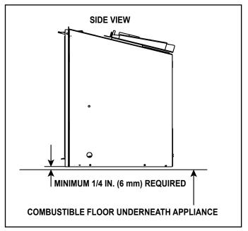
Figure 3.17 Solid Fuel Floor Clearance
