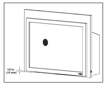
Figure 9.5 Required 1/2 in. (13 mm) Gap
