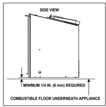
Figure 3.4 Solid Fuel Floor Clearance
