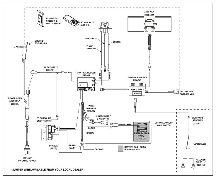
→ Figure 6.2 IntelliFire<sup>™</sup> Plus Wiring Diagram with Remote
