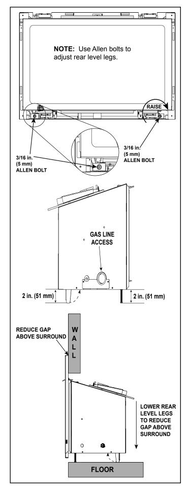
Figure 5.13 Leveling Leg Detail
