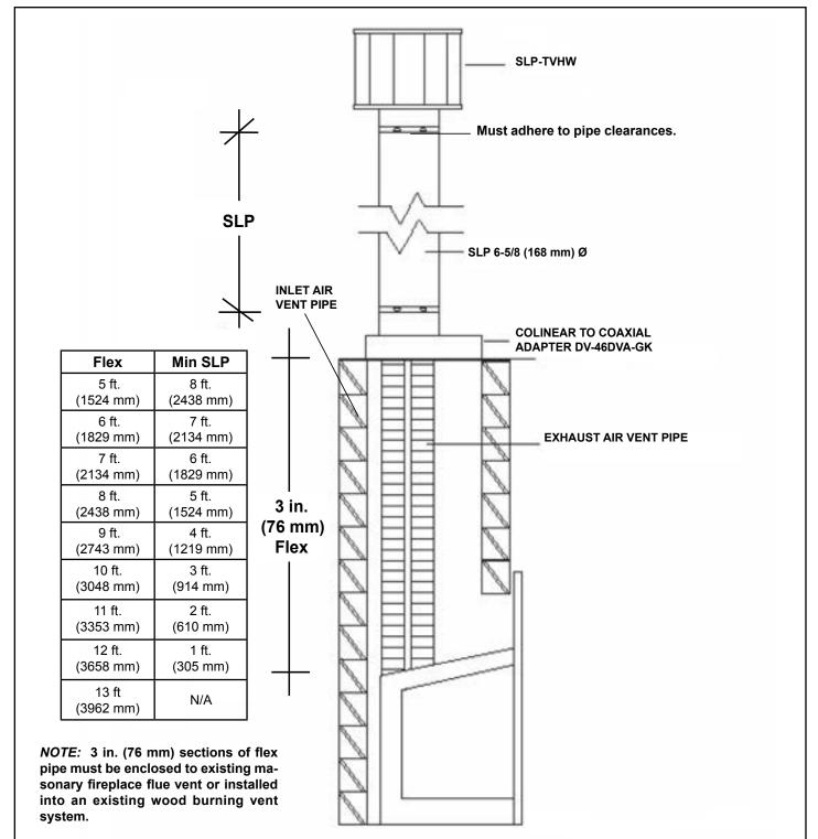
Four 45 degree elbows can be used in the vertical section of SLP venting to avoid structural members such as floor joist or trusses. Maximum total vent run is 50 ft (15.24 m). 90 degree elbows may NOT be used.
