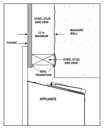
Figure 3.10 Transition Sealing Detail for Wall Extensions (Side View)
