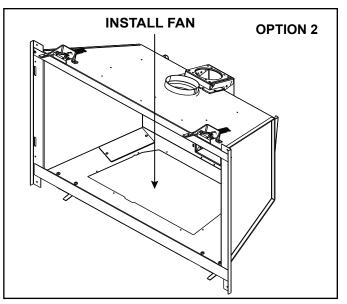
Figure 6.4 Through Valve Plate Opening (Option 2)
