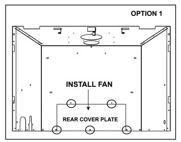
Figure 6.3 Cover Plate Removed (Option 1)
