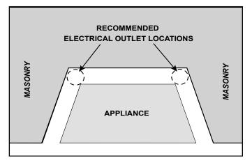
Figure 4.2 Electrical Outlet Detail
