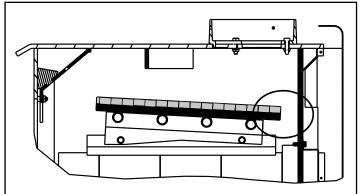
Ceramic Blanket and Baffle Board are NOT in contact with the back of the firebox.
