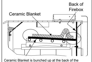
firebox and NOT even with the Baffle Board in the front.
