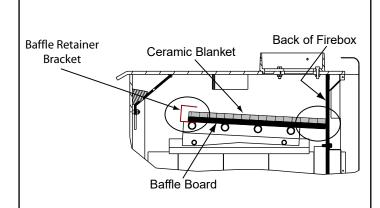
Ceramic Blanket and Baffle Board MUST be in contact with the back of the firebox and even with each other in the front.
