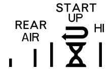
After activating the timer (ACC), if the control is placed within the rear air section on the label it will allow rear air to enter the firebox. This will not interfere with the timer gradually closing the front air channel in 25 minutes. If control is set on "HI" it over-rides the timer (ACC).
