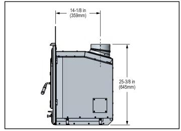
**Figure 3.8** - Side View with Flat Surround and Optional 15 Degree Adapter (DV-6DLR-E15ADSS)
