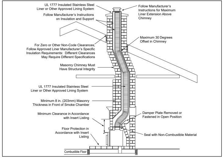
Figure 4.3 - Generic Insert Model Shown in Illustration
