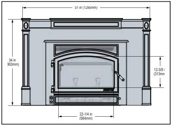
**Figure 3.6** - Front View with Large Flat Surround (CT2-5134) with Cast Trim (811-0930)
