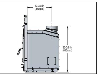
**Figure 3.11** - Side View with Cast Surround and Optional 15 Degree Adapter (DV-6DLR-E15ADSS)
