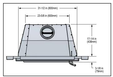
Figure 3.4 - Top View with Cast Surround
