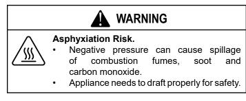
Negative pressure results from the imbalance of air available for the appliance to operate properly. It can be strongest in lower levels of the house.
