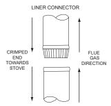
Figure 14.1 - Chimney Connector (Appliance Pipe)
