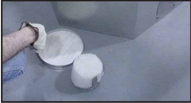
Figure 28. Discard the flue cap, remove and discard the insulation basket. Note: Once the flue cap has been removed it CANNOT be reattached.
