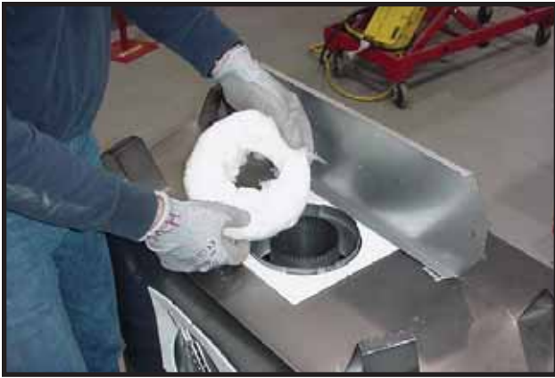
Figure 23. Remove the insulation from the outer flue pipe.
