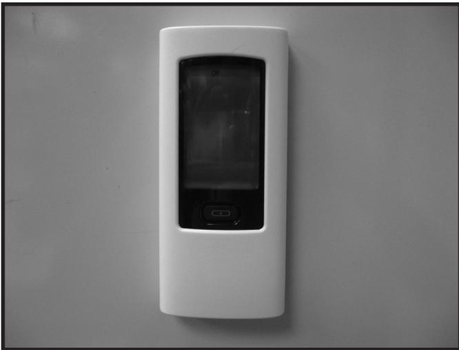
Figure 12.6 Mounting Remote Control Housing
