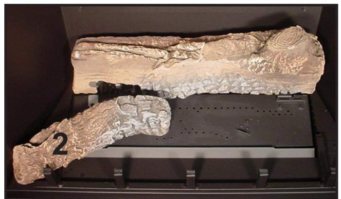
**LOG #2 (SRV2033-701):** Locate the bottom groove of log #2 over the left most grate tine and align over the burner by placing the log slot over the burner tab as shown.
