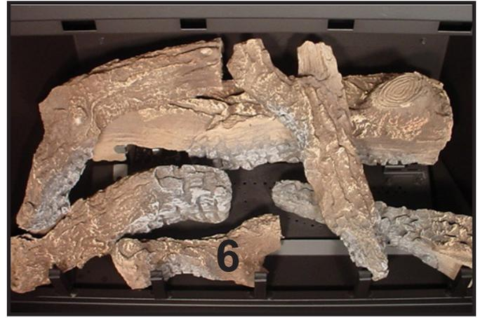
**LOG #6 (SRV540-704):** Place log #6 against the second and third grate tines. If sooting occurs, the logs might need to be repositioned slightly to avoid excessive flame impingement.
