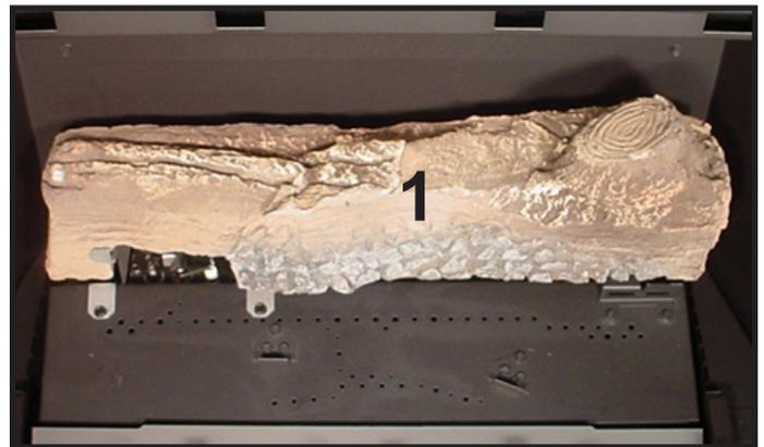
**LOG #1 (SRV327-701):** Place log #1 at the rear of the unit, with the left edge behind the tab on the pilot bracket. The right side sits behind the tab on the support bracket.
