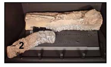
**LOG #2 (SRV2033-701):** Locate the bottom groove of log #2 over the left most grate tine and align over the burner by placing the log slot over the burner tab as shown.
