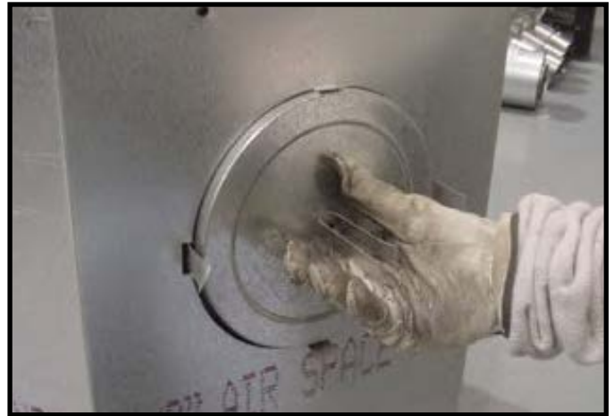
Figure 6.10 (Generic Appliance Shown) Fold the center parts of the retaining band out and use to remove the seal cap.
