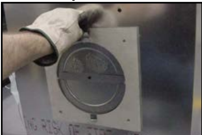
Figure 6.8 (Generic Appliance Shown) Fold the tabs toward the center of the fire plug (90°) and remove the insulation gasket.
