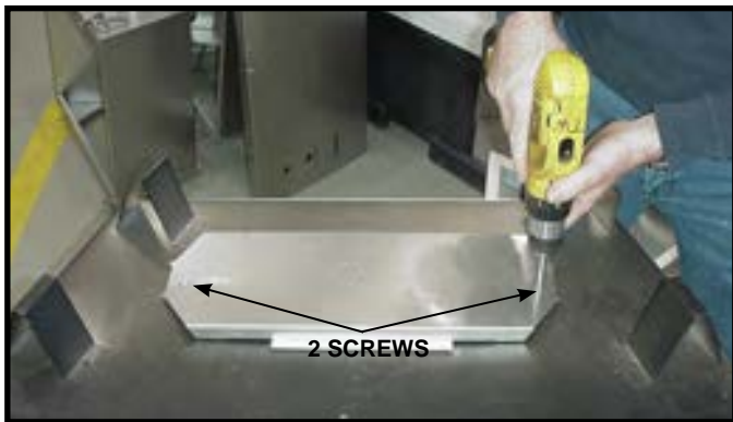
Figure 6.1 For top vent, remove the two screws holding the top heat shield in place. For rear vent, see next page.
