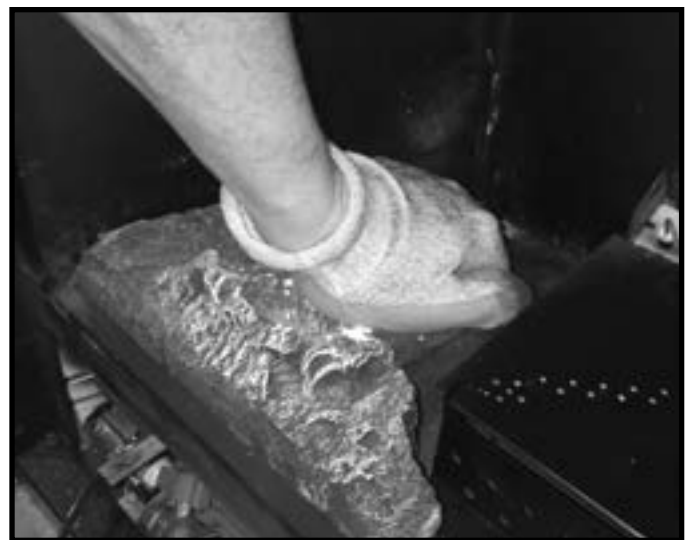
Figure 11.2 Press Left Hearth Firmly Into Place
