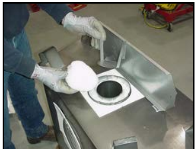
Figure 6.5 Remove the insulation basket and white insulation from the center vent pipe.
