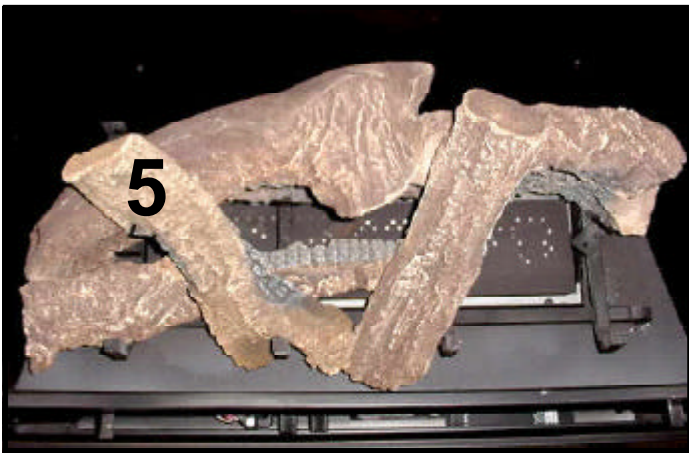
LOG #5 (SRV347-702): Put the forked end of log #5 over the second vertical bar and rest the top end to the right of the grooved section of log #1.
