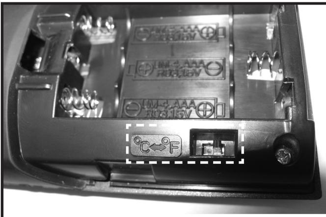
Figure 12.3 Temperature Scale
