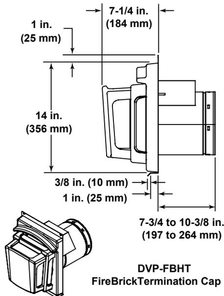
Figure 16.4 DVP vent components
