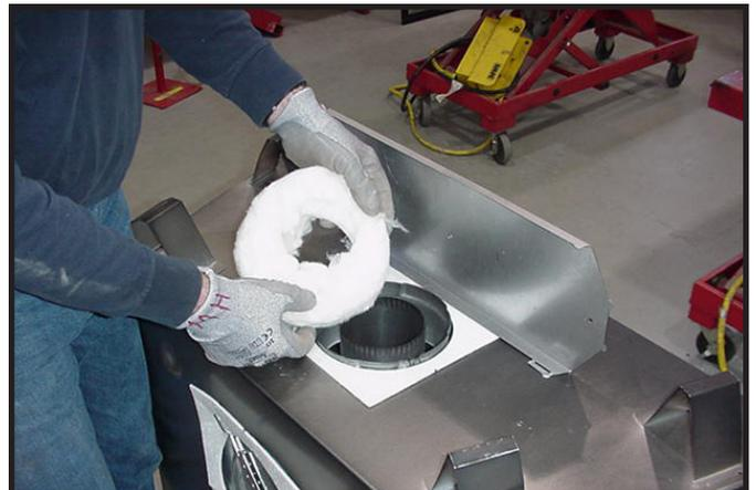
**Figure 9.6** Remove the insulation from the outer vent pipe.
