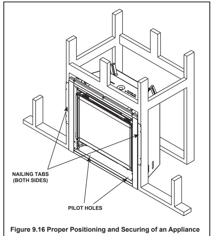
**Figure 9.16** Proper Positioning and Securing of an Appliance
