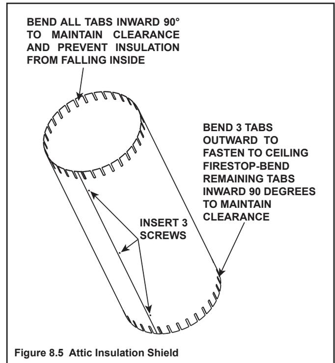
Figure 8.5 Attic Insulation Shield
