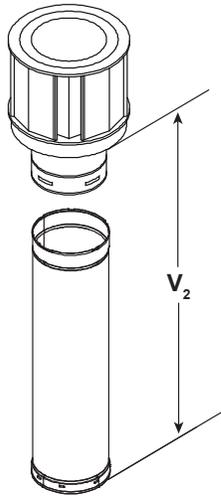
**Note:** A 6 in. (152 mm) section of straight flue must be attached to the heater before a 90° elbow.
