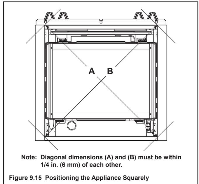
**Note:** Diagonal dimensions (A) and (B) must be within 1/4 in. (6 mm) of each other.
