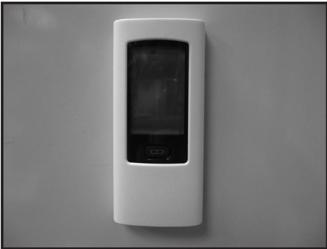
Figure 12.6 Mounting Remote Control Housing
