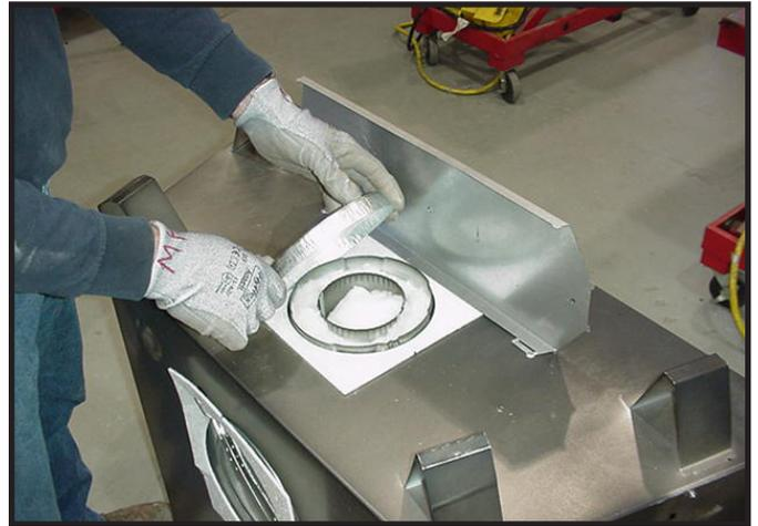
**Figure 9.4** Remove the seal cap.
