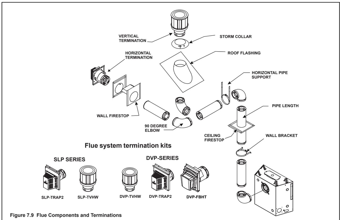
Figure 7.9 Flue Components and Terminations
