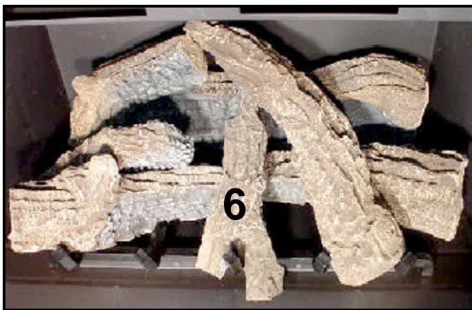
LOG #6 (SRV438-724): Place the "Y" shaped part of log #6 over the 3rd grate bar. Rest the tip of the log against log #1 and log #5.
