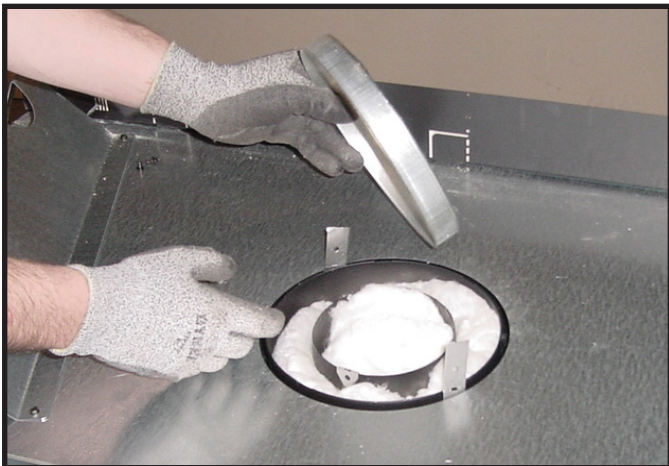
Figure 9.3 Remove the seal cap.
