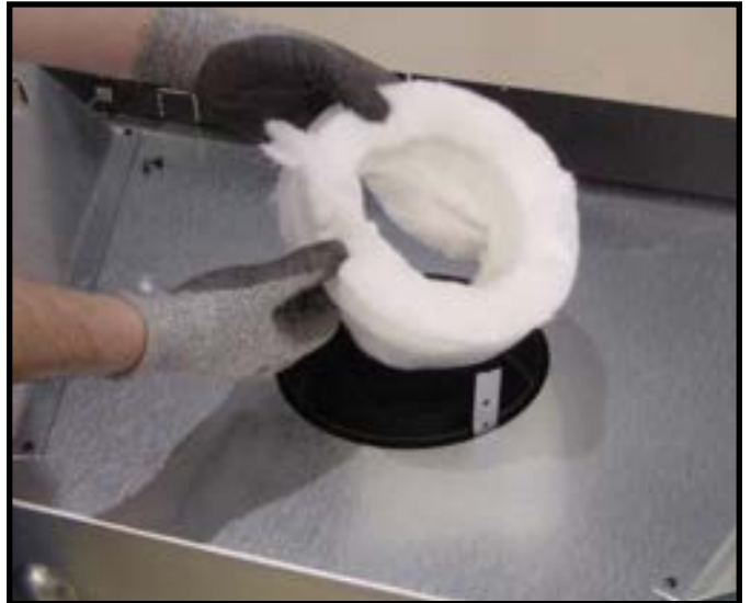
Figure 6.5 (Generic Appliance Shown) Remove the insulation from the outer vent pipe. For rear venting there is no insulation in the outer vent pipe.
