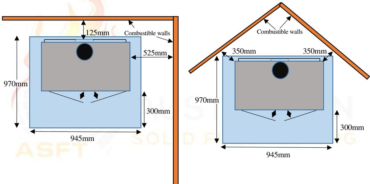
Figure 1 – Clearance Diagram
