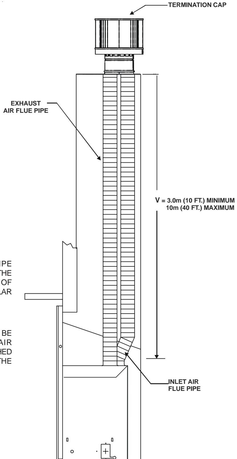
**WARNING:** THE EXHAUST PIPE MUST ONLY BE CONNECTED TO THE EXHAUST STARTING COLLAR OF THE UNIT AND THE CENTER COLLAR OF THE TERMINATION CAP.
