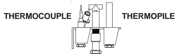
6. To put the control in the pilot position, turn the control knob counter-clockwise
