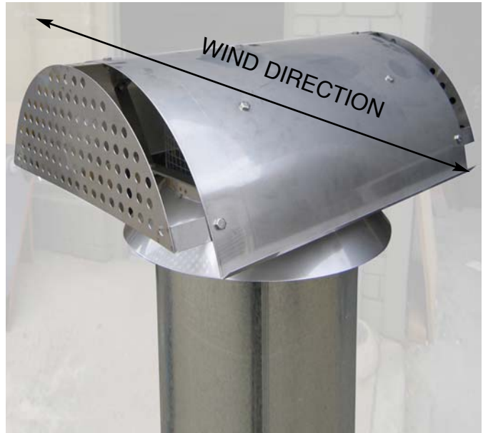
FIX COWL TO TOP OF FLUES, WITH ROUNDED TOP EDGE FACING AGAINST PREVAILING WIND
