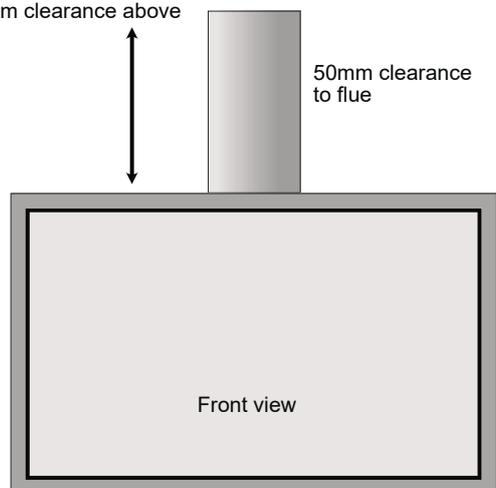
Zero clearance required under the casing
