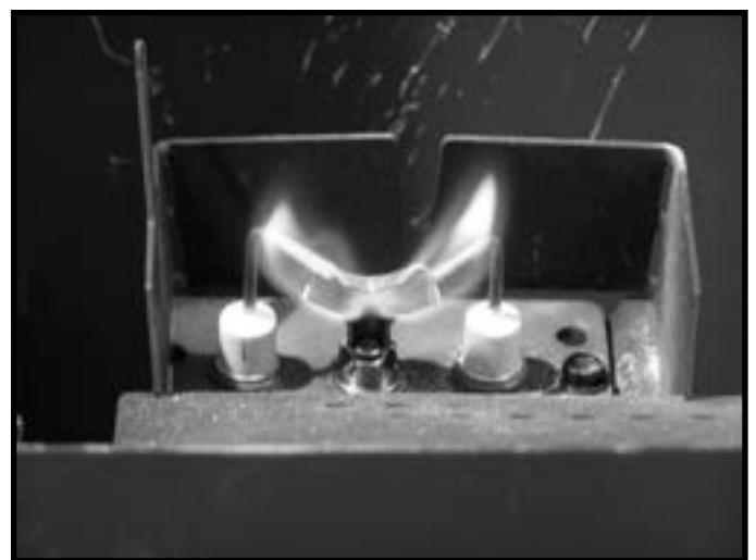
Figure 4.2 IPI Pilot Flame Patterns
