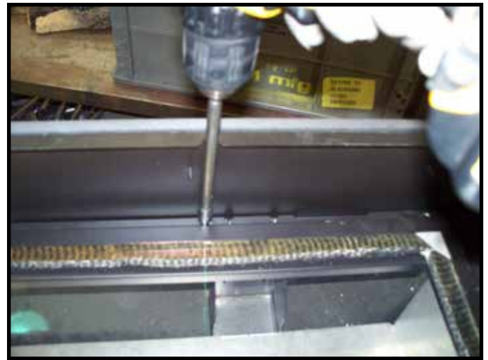
Figure 9.4. Gas and Electrical Access - Remove Glass Window
