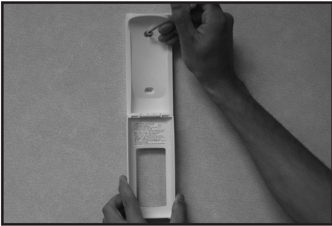
Figure 3.8 Mounting Remote Control Housing
