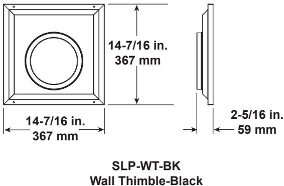
Figure 12.2 SLP Series Vent Components
