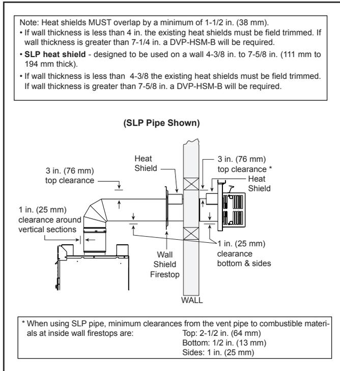
Figure 5.1 Horizontal Venting Clearances To Combustible Materials
