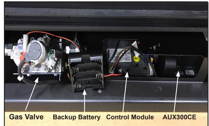
Figure 8.2 Gas Valve, Backup Battery, Control Module & AUX300CE
