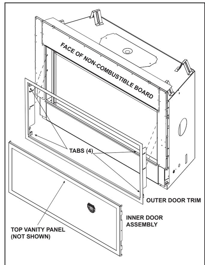
Figure 10.9 CFTF Front Installation With Outer Door Trim
