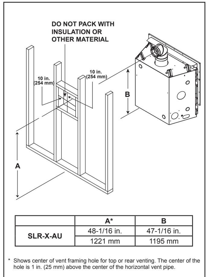
Figure 5.2 Wall Penetration
