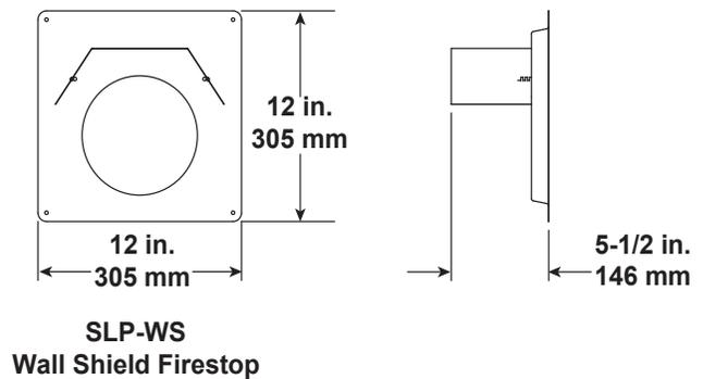
Figure 12.1 SLP Series Vent Components
