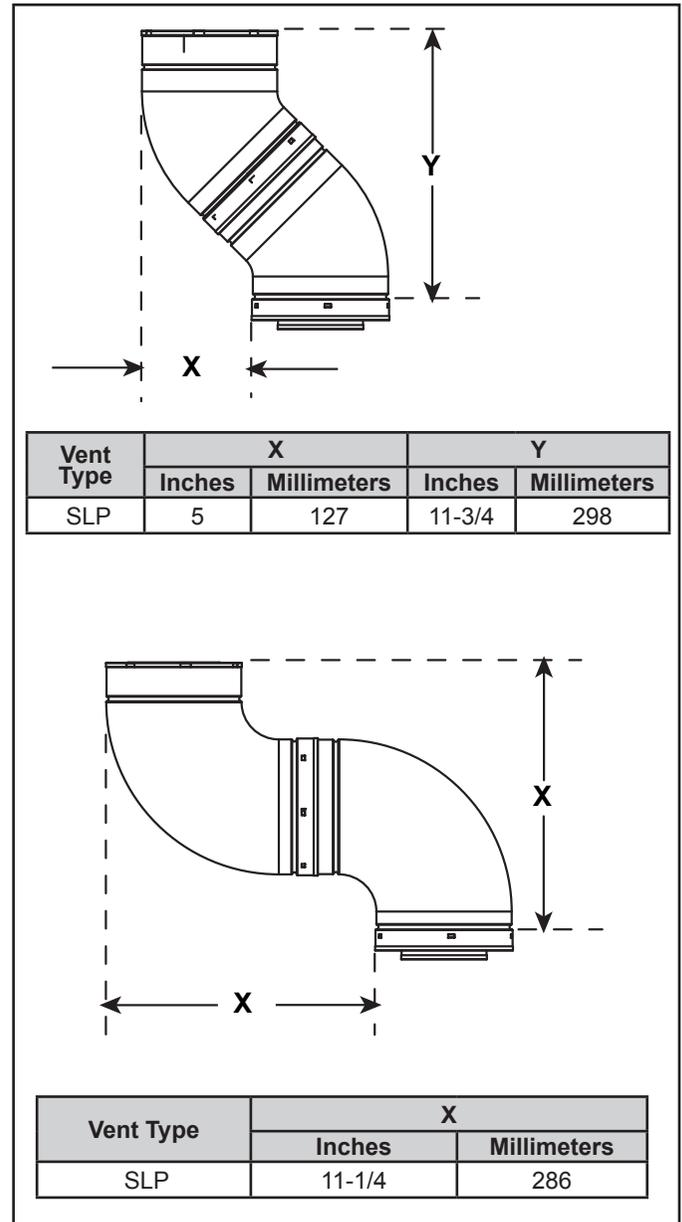
Figure 4.5 Vertical and Horizontal Offset for SLP Elbows
