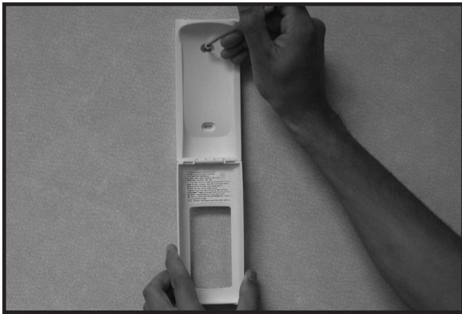
Figure 3.8 Mounting Remote Control Housing
