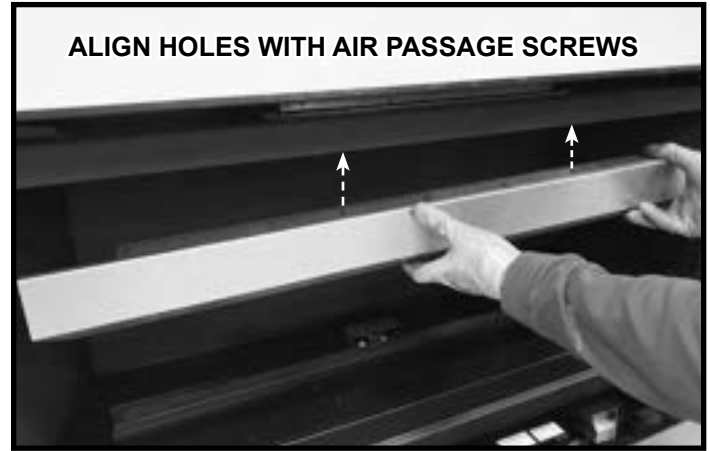
Figure 12. Glass Baffle Alignment
