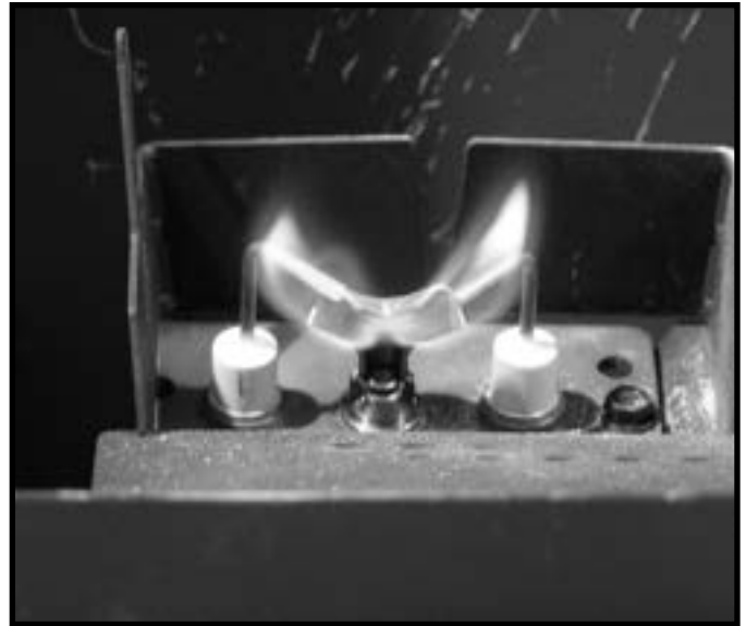
Figure 4.2 IPI Pilot Flame Patterns
