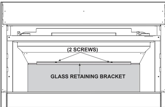
Figure 3. GLASS-36LINEAR: Back Glass Retaining Bracket Installed
