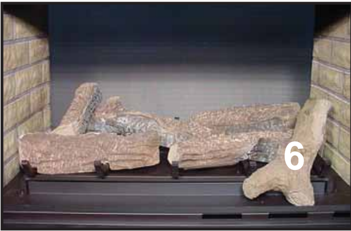
LOG #6 (SRV582-705): Position log #6 on top of the groove in log #3 with the forked end resting on the grate assembly as shown.
