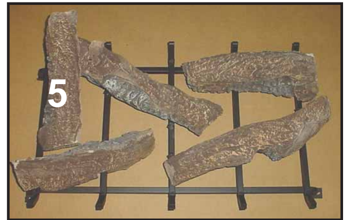
LOG #5 (SRV2068-703): Place log #5 on top of flat spot on log #1 and against the inside of log #2. Be careful not to reposition log #2 when placing this log.
