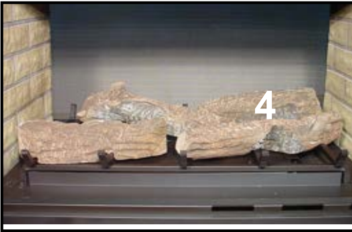
LOG #4 (SRV2068-703): Place log #4 in the right rear corner of the log grate using bottom grooves for placement. Align log #4 by using the grate corner and rear cross bar as stops.
