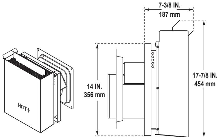
Figure 14.4 - SLP Series Vent Components
