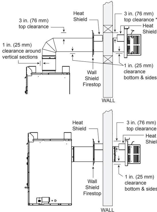
\* When using SLP pipe, minimum clearances from the vent pipe to combustible materials at inside wall firestops are:
