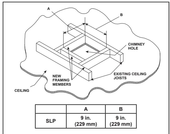
Figure 10.13 - Hole and New Framing Members
