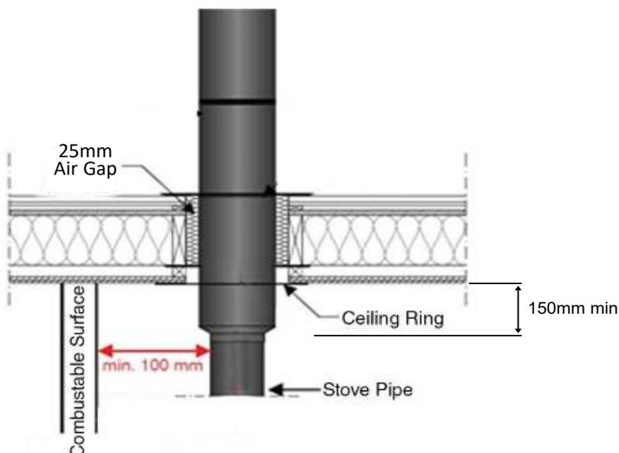
Once in desired position, tighten off the flue brace bracket and use self-tap screws (not supplied) to fix off the Safety Vent AIR pipe. The 25mm gap between a combustibile ceiling and the Safety Vent AIR pipe can be covered using the 80mm steel ceiling ring flush to the ceiling with no airgap required. (FIG 3)
