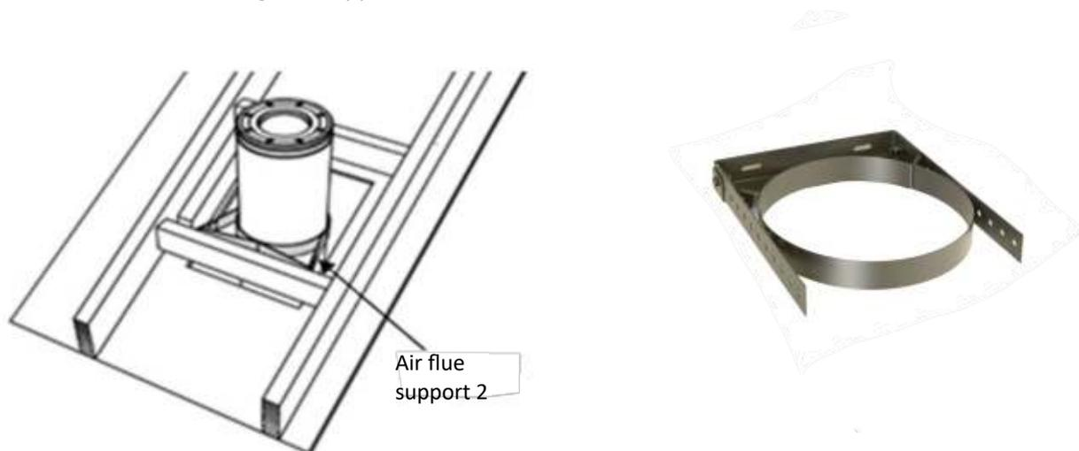
At the roof level, use appropriate flashing to weather seal the penetration. (Not supplied)
