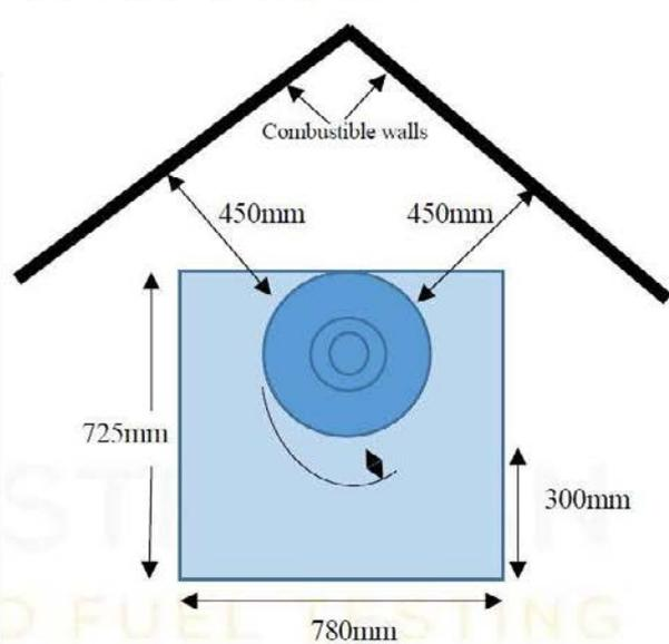
\* The appliance can spin 360 degrees on its base. Therefore, when the front of appliance faces a combustible wall, the minimum 1500mm clearance to combustible surfaces must be maintained. A minimum forehearth clearance of 300mm must be maintained in front of the appliance.
