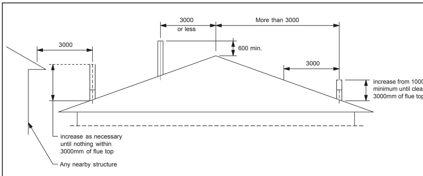
**Figure 16.1 Minimum Height of Flue System Exit**
