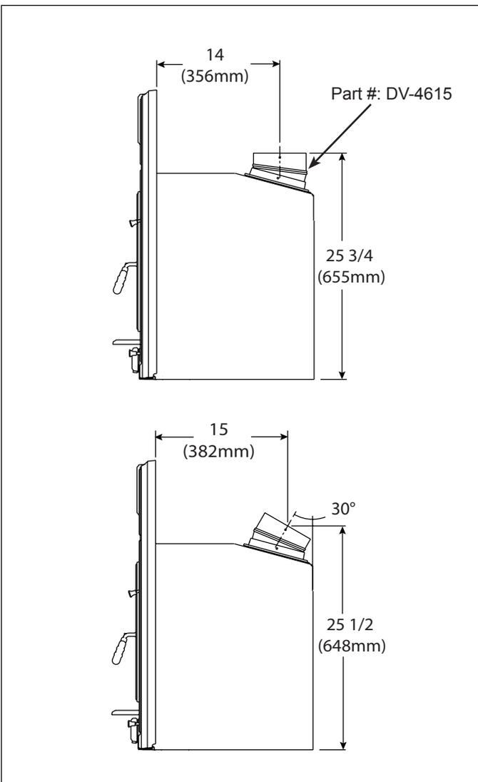
**Figure 12.3 - Side View With Optional Flue Adapter**
