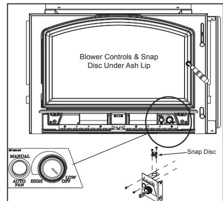
**Figure 7.1 Snap Disc Location**
